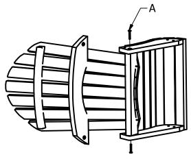
**1)** Insert an A bolt into lower hole to on each side attach Seat to Back. Make sure the back is fully upright. Make bolts snug, but do not overtighten.
